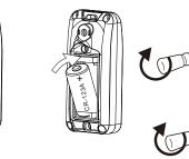
Insert a CR123A battery and replace the battery cover
